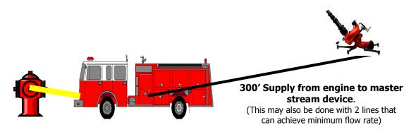
**Objective:** Establish a portable master stream attack utilizing 300' of supply hose or 2-3" lines of equal length. A minimum of 500 GPM must be flowing from nozzle. Tank water may be used until the hydrant supply is established. A maximum of 10 seconds of interruption in flow is allowed during transfer from tank water to positive pressure source.
